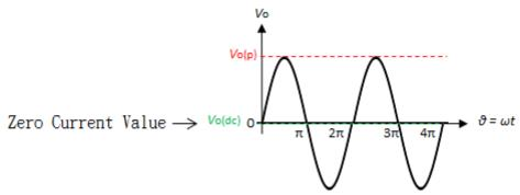
Figure 1 The zero current value of sine waveform
