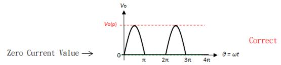
Figure 3 The zero current value of the asymmetric waveform (Correct)
