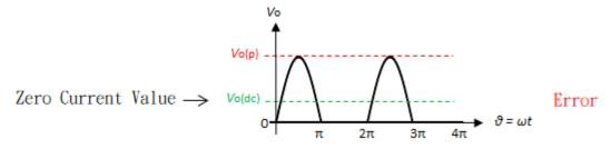
Figure 2 The zero current value of the asymmetric waveform (Error)
